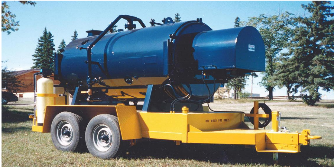
Fig.2. 5. A portable boiler
