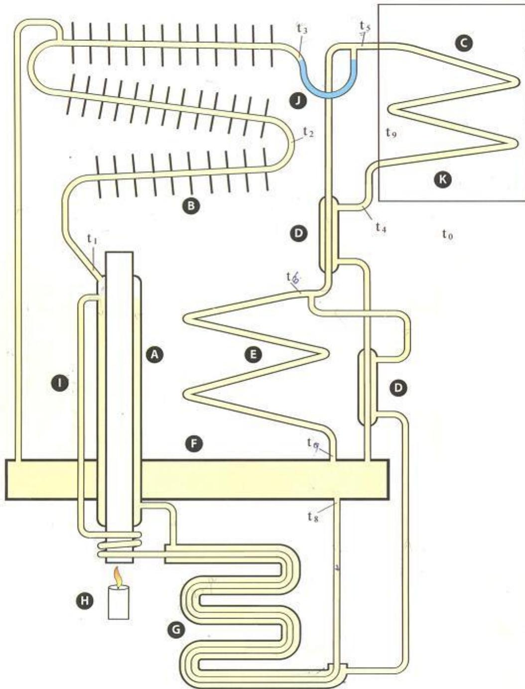
Figure 3.1: Schematic diagram of Electrolux Refrigerator
