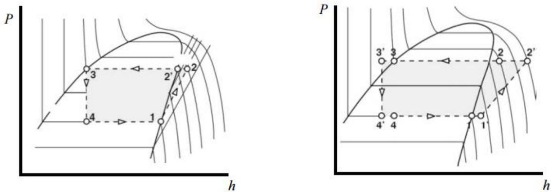
Figure 1.1: Pressure-enthalpy diagram of an (a) ideal refrigeration cycle (b) real refrigeration cycle
