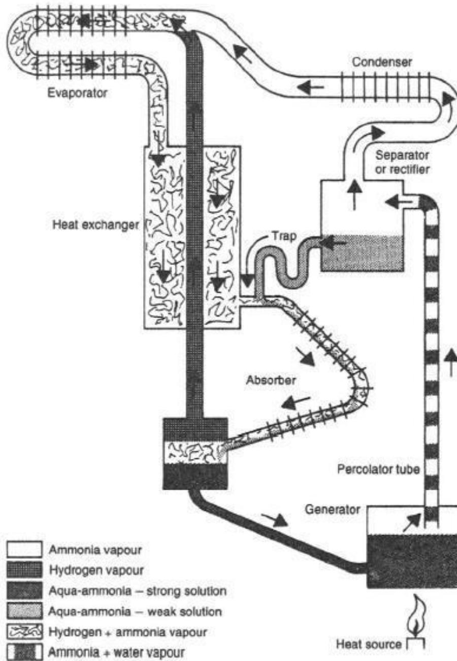
**Figure** Absorption system cycle
