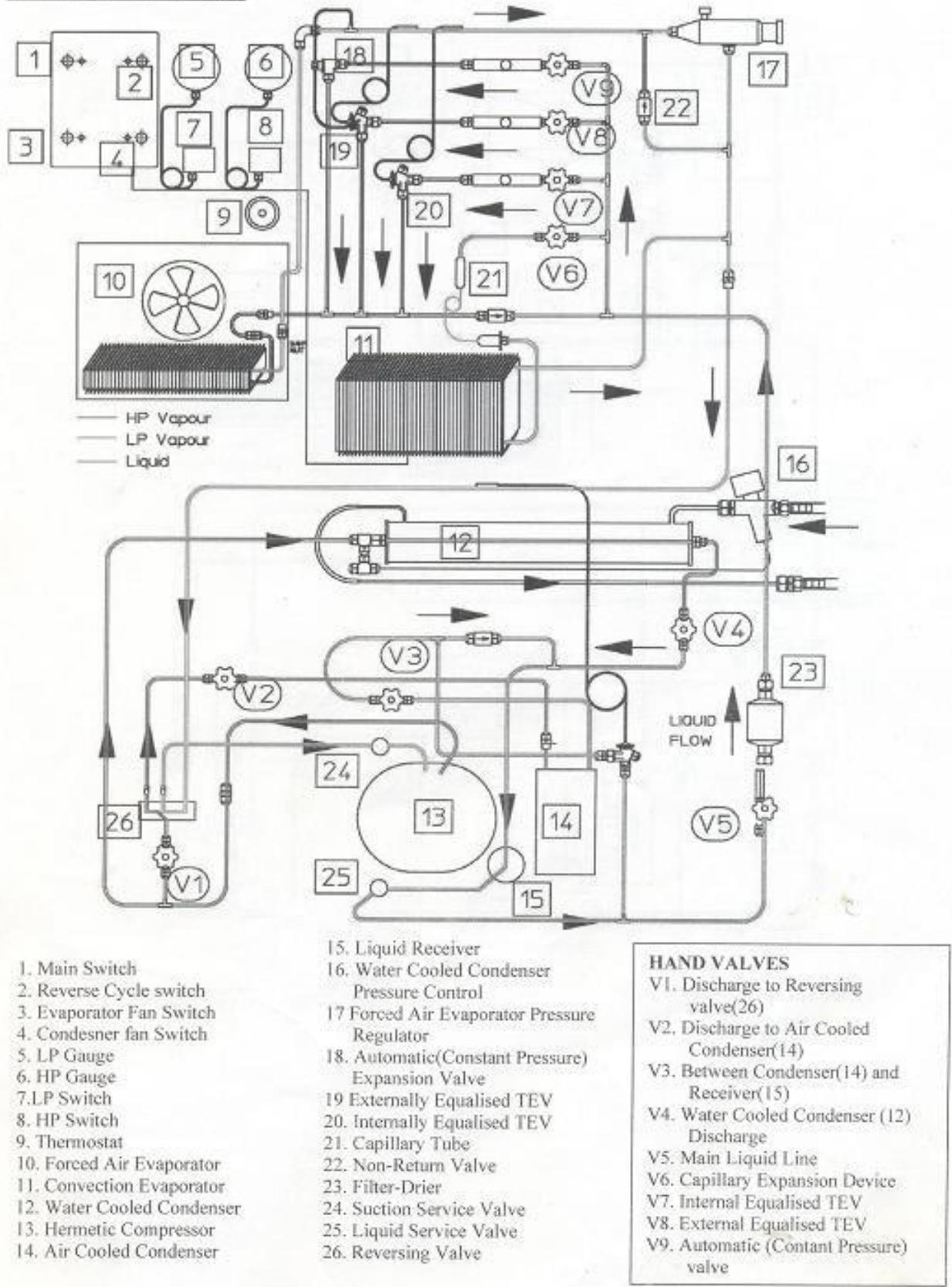
**Figure 5.2: Normal operation Schematic diagram**
