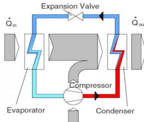
Figure 1.2: Vapor Compression Refrigeration Cycle
