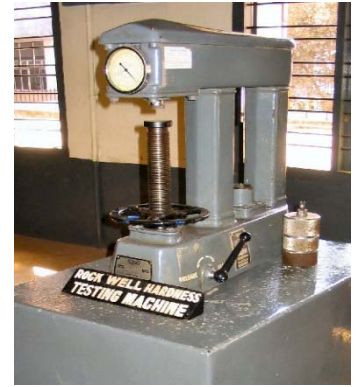
Figure 9- 1 Rockwell Hardness Testing Machine
