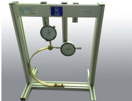
Figure 7- 1Semi Circular Curved Bar Apparatus
