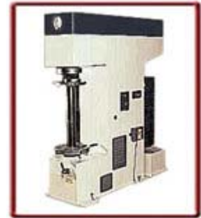
Figure 9- 4 Brinell Hardness Testing Machine
