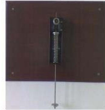
Figure 1- 1 Compression spring apparatus
