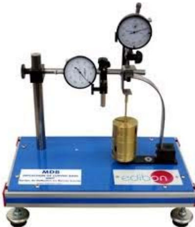
Figure 6- 1Quarter Circular Curved Bar Apparatus
